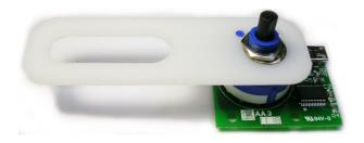
Fit collar onto handle and switch. Tighten screws using supplied allen key.
