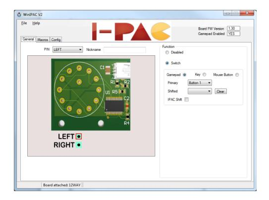
On the Config tab, there is a setting for "Switch Debounce". This can be set to one of 4 settings. On this interface, this controls the length of the key "pulse" issued on each click. Some slower applications may require a longer pulse.
