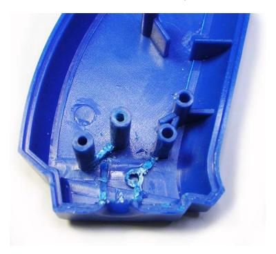
The charging PCB should fit right down to the base, so the connector lines up with the hole.
