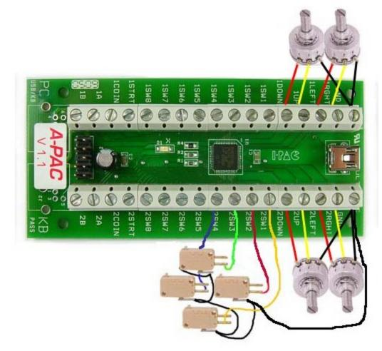
The "Start1" input changes the selected buttons to the shifted set, buttons 13-28 in Windows. This behaves in exactly the same way as the I-PAC shift button. All the other inputs are ordinary buttons.
