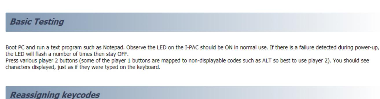
This is done using WinIPAC V2. For full instructions, click the Configuration Utility tab. I-PAC boards support left/right mouse buttons plus game controller buttons, volume up/down, power, sleep and wake, in addition to keyboard keys. Extensive macro support is available.
