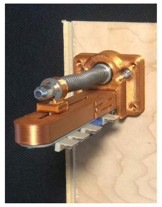
Make sure not to overtighten and damage the plunger housing plate. Screws should be tight enough to hold the ball shooter in place but not so tight as to split mounting plate. If the angle of the plunger is too high toward the front, put the supplied panhead wood screws into the bottom holes of the plunger and tighten to bring down the nose of the plunger.
