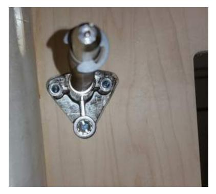
Mount plunger using supplied machine screws and star washers (washers not really necessary).
