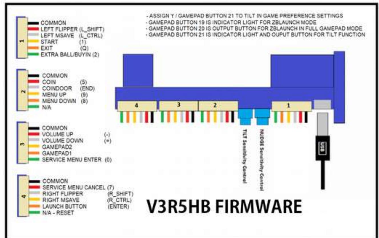
The plunger is hardcoded for the Standard button layout for Visual Pinball. Additionally, there are 2 gamepad buttons available to be assigned to any function not covered by the hardcoded keystrokes in keyboard mode.
